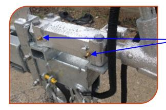
Grease Point on Tow Hitch Grease on regular basis
